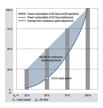
**Reduced energy consumption:** The bars show the power consumption of fans that are switched on stepwise as needed. Air performance is reduced by 50 % when half of the fans are switched off. The blue line shows the power consumption of all fans with smooth speed adjustment at the required air flow (50 % air flow = only 12.5 % input power).
