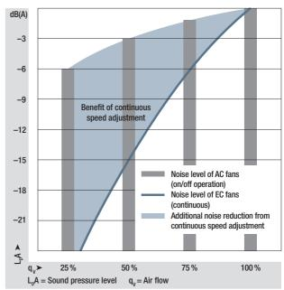
**Lower noise generation:** While switching off half the fans (50 % decrease in air flow) only reduces noise generation by approx. 3 dB, a speed reduction resulting in 50 % less air flow achieves an improvement of 15 dB.
